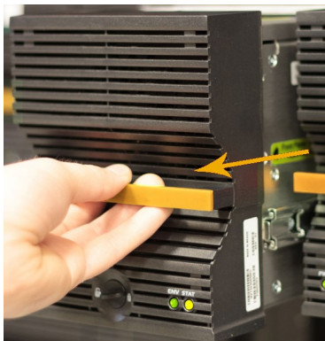
Figure 3-6: Sliding the drive drawer out
