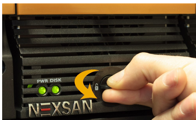
Figure 3-5: Unlocking the drive drawer
