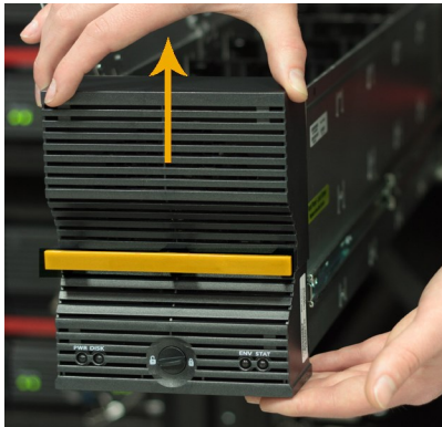
Figure 3-10: Removing the drawer front assembly
