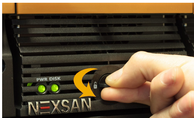
Figure 2-4: Unlocking the drive drawer
