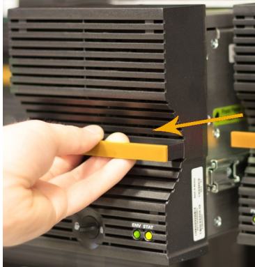
Figure 2-5: Sliding the drive drawer out
