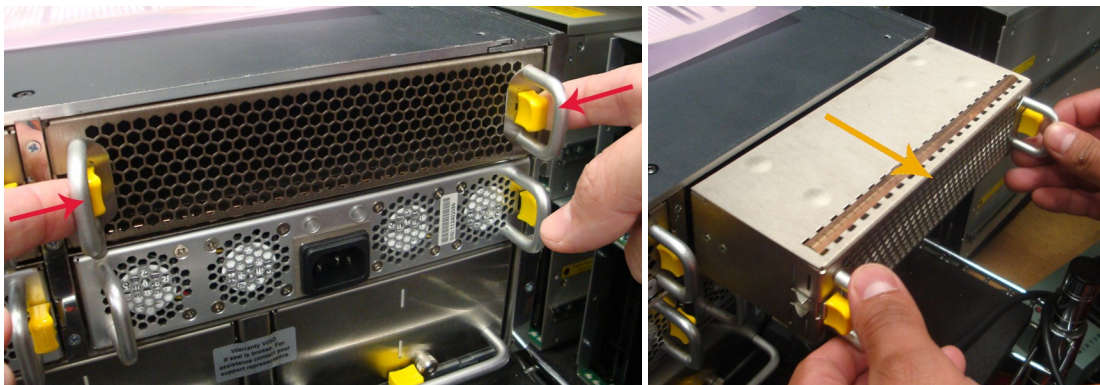
Figure 2-2: Removing the back plate
