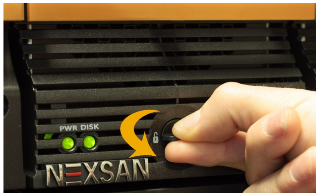
Figure 2-2: Unlocking the drive drawer
