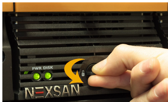
Figure 3-5: Unlocking the drive drawer
