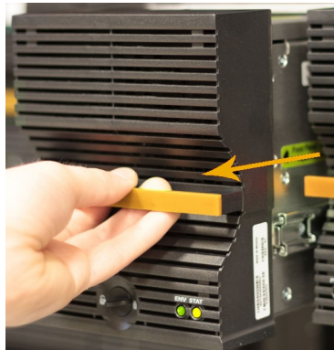
Figure 2-3: Sliding the drive drawer out
