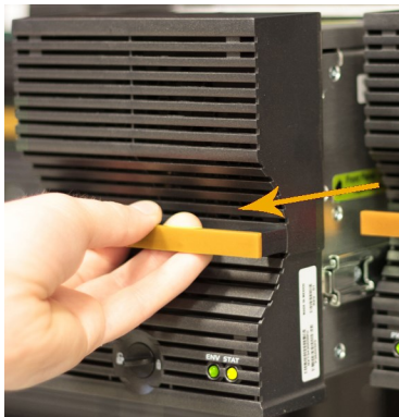
Figure 3-6: Sliding the drive drawer out
