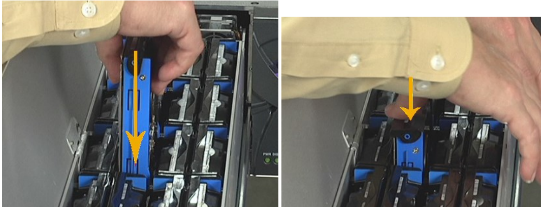
Figure 3-8: Loading a new disk drive
