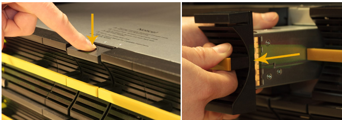
Figure 3-15: Removing the central fan assembly
