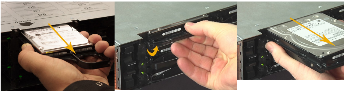
Figure 3-7: Removing a disk drive (Nexsan E32, left; Nexsan E18, middle and right)
