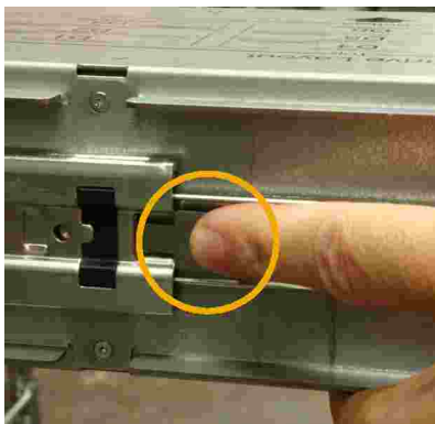
Figure 3-15: Disengaging the drawer side-rail latch
