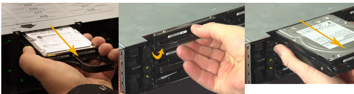
Figure 3-7: Removing a disk drive (Nexsan E32X left; Nexsan E18X, middle and right)
