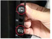
2. Loosely attach the rear mounting brackets to the rear of the rack, then screw two flanged-head screws into the sides of each bracket. Be sure to leave approximately 1mm of thread showing.
