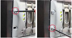
6. Tighten the screws holding the rear mounting brackets to the rack, then tighten the screws on the sides of the mounting brackets to secure the mounting rails.
