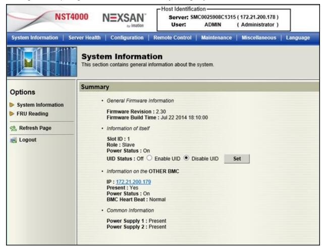
6. To launch a remote session to the Unity Storage System, click the **Remote Control**button at the top of the IPMI Web-based interface's main screen. This opens the Remote Control page.
