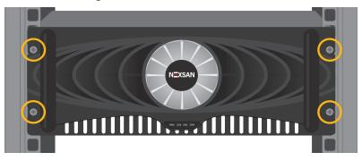
2. Carefully slide the unit for ward on the rails until the bolts securing the front panel to the unit are visible.
