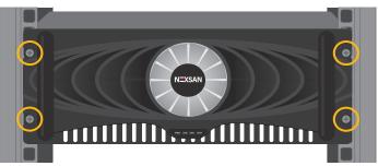
4. Carefully slide the unit for ward on the rails until the side rail latches click into place.
