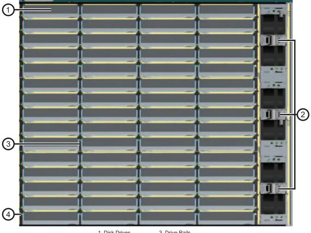
1. Disk Drives3. Drive Rails2. Rear Fan Assemblies4. Drive Status LEDs
