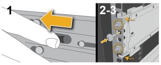
3 Using the four supplied silver bolts, bolt the front and back of each rail to the rack posts. NOTE: The rails should be installed into the middle 2U of the 4U of rack space where you wish to install the BEAST. For example, if you want the BEAST to occupy U slots 18 through 21, install the rails into U slots 19 and 20.
