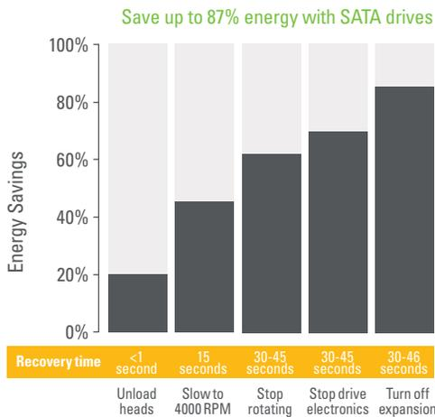
Lastly in video surveillance, the storage system can be configured with 7 RAID disk sets, one for each day of the week. In this configuration only one RAID disk set needs to be powered up at any given time to accept that day's data, resulting in startling power savings. Of course all drives are accessible as needed, should someone wish to view or process the video captured on prior days.
