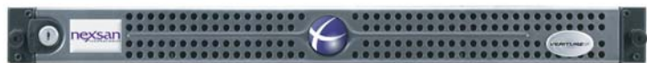
Nexsan's Veriture-iP lets users attach SCSI RAID arrays to a Gigabit Ethernet network.
