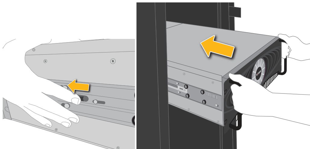
Figure 3-5: Disengaging the side rail latches and sliding the Nexsan Storage System into the rack
