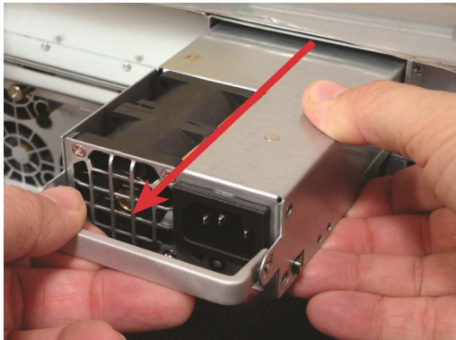
Figure 1-31: Removing the PSU
