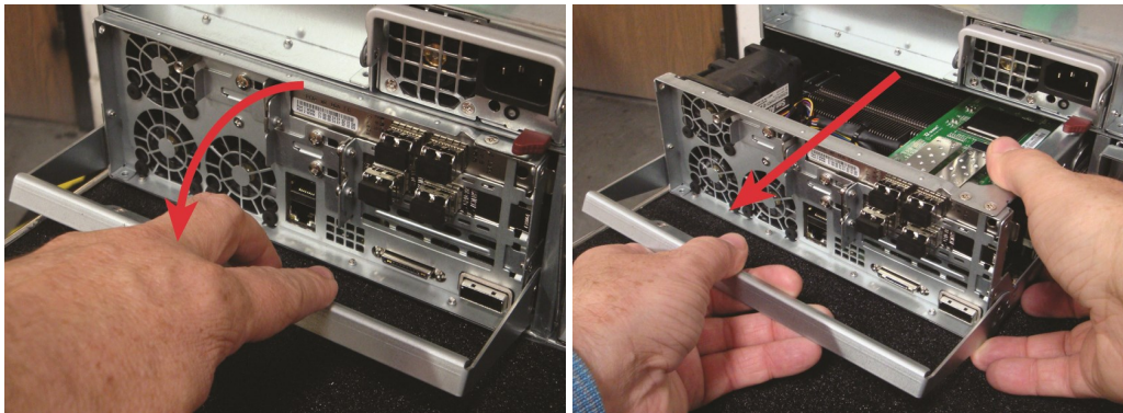
Figure 3-2: Removing the Unity Storage System controller
