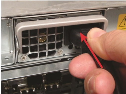
Figure 1-33: Applying power to the PSU
