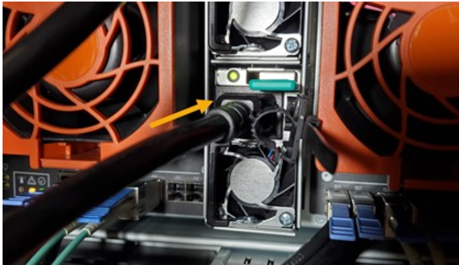
Figure 1-37: Applying power to the PSU
