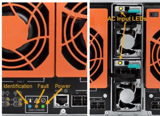
Figure 1-26: U2G460 rear power LED (left) and rear AC Input LEDs
