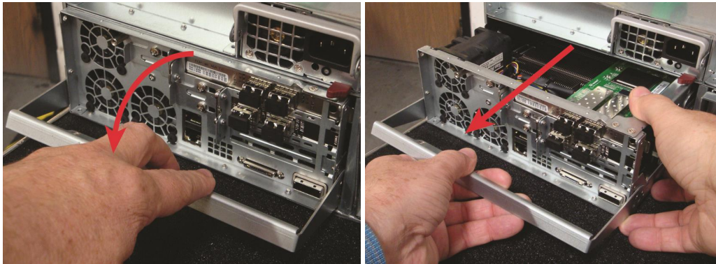
Figure 3-2: Removing the Unity Storage System controller
