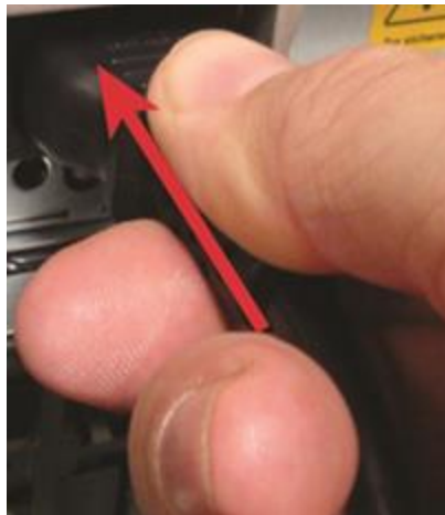
Figure 1-33: Applying power to the PSU
