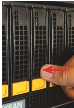
Figure 1-15: Latching the new disk into place
