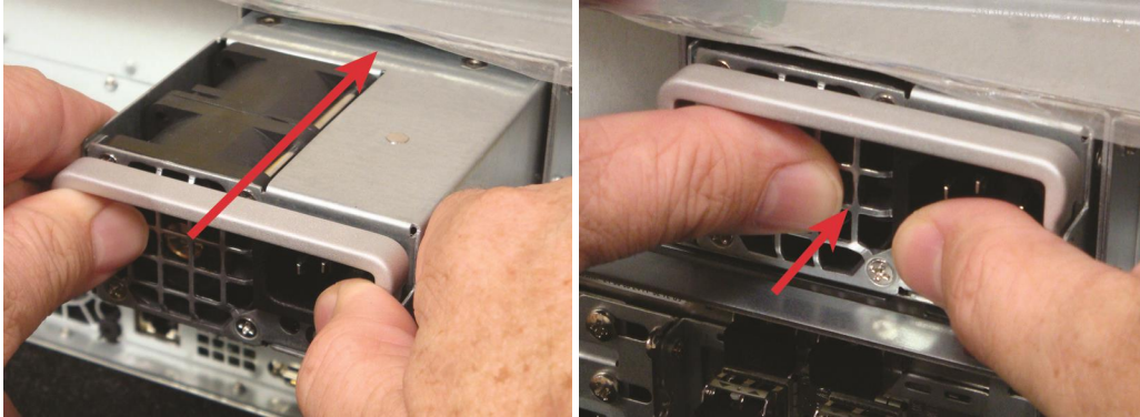
Figure 1-29: Installing the new PSU
