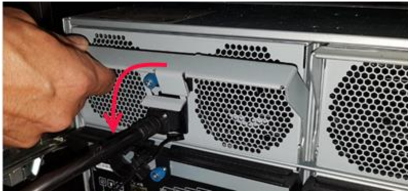
Figure 1-32: Unlatching the PSU
