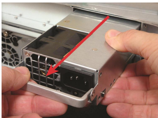
Figure 1-28: Removing the PSU
