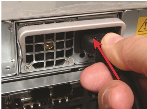
Figure 1-30: Applying power to the PSU
