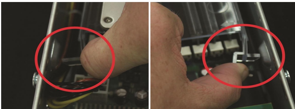
Figure 5-12: Removing the plastic shelf
