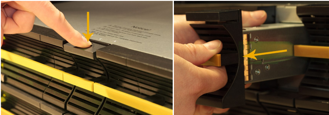
Figure 3-15: Removing the central fan assembly
