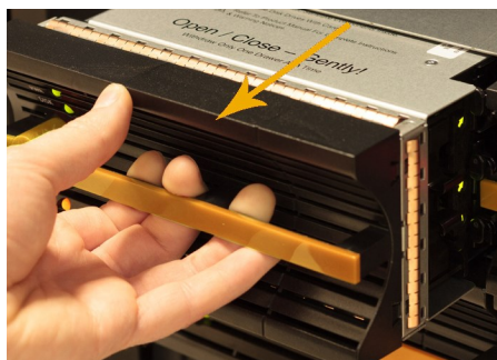
Figure 2-3: Sliding the drive drawer out
