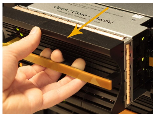
Figure 3-6: Sliding the drive drawer out
