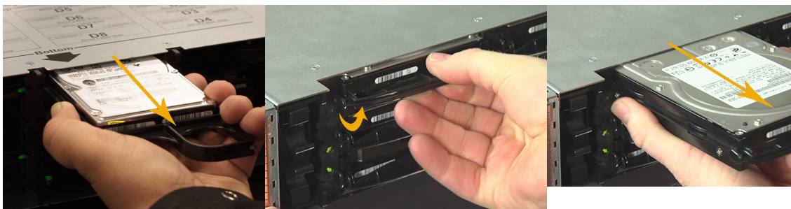
Figure 3-7: Removing a disk drive (Nexsan E32X left; Nexsan E18X, middle and right)
