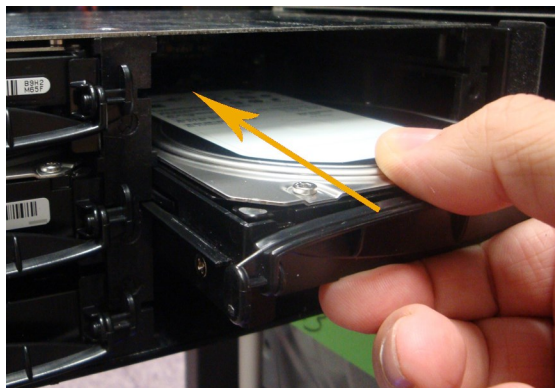
Figure 2-4: Loading a new disk drive (Nexsan E18X top; Nexsan E32X bottom)
