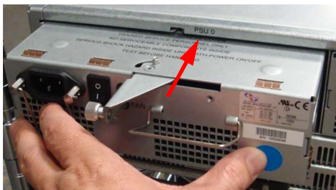
Figure 4.2: Sliding the PSU into place
