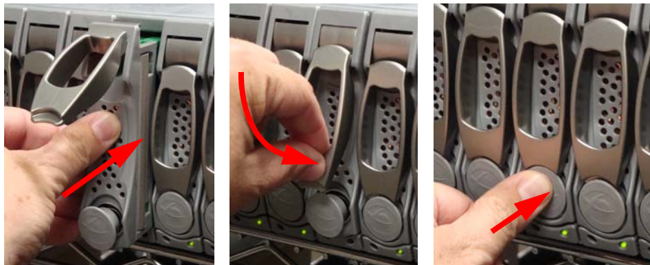
Figure 4.9: Replacing a disk drive
