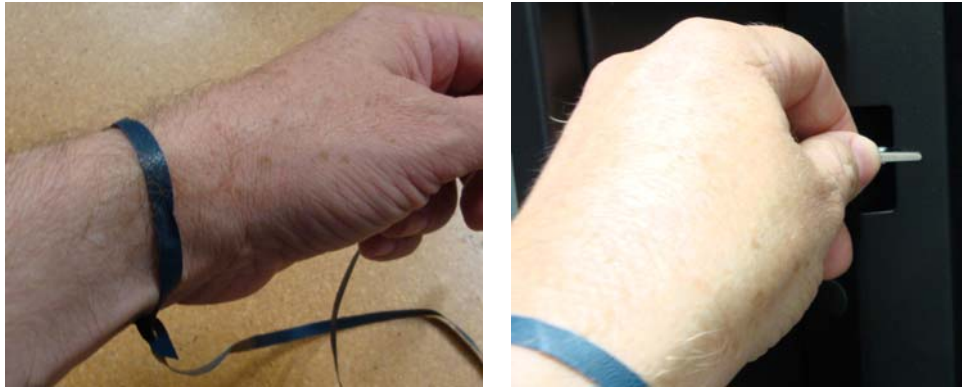
Figure 3.1: Putting on and attaching the anti-static wrist-strap.
