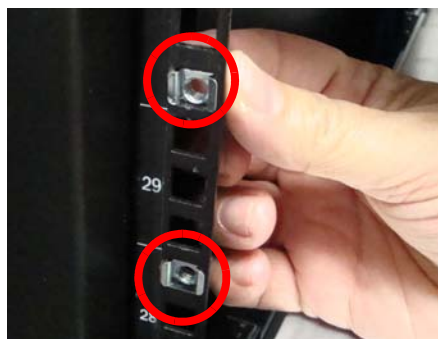
Figure 2.5: Attaching the cage nuts
