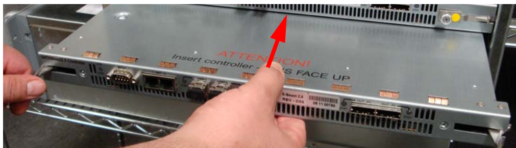
Figure 4.5: Sliding the RAID Controller into place
