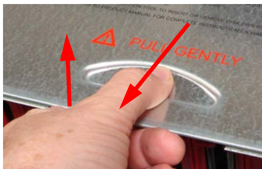
Figure 4.11: Opening the drive bay lid
