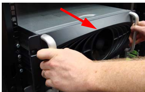
Figure 3.14: Sliding the unit forward in the rack
