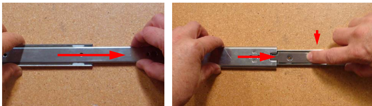
Figure 2.9: Separating the inner and outer side rails
