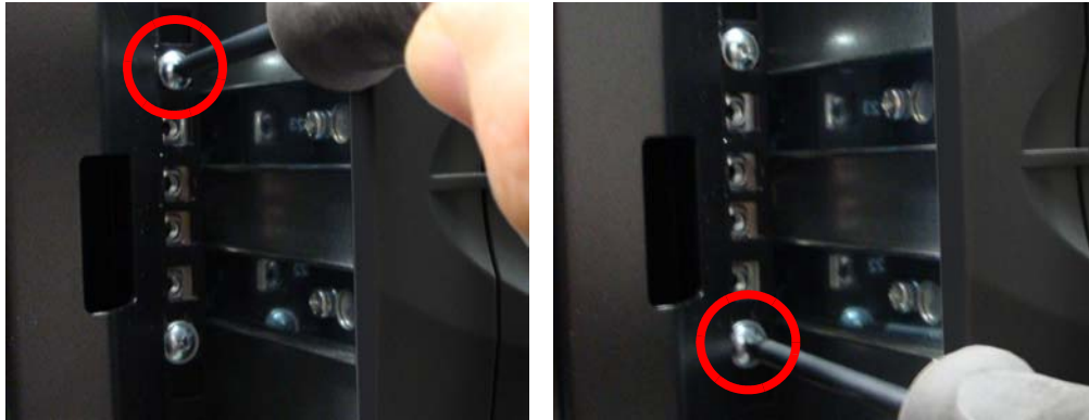
Figure 3.7: Tightening the front rack mount screws
