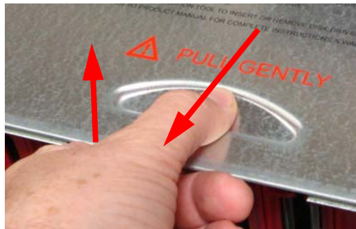
Figure 3.16: Opening the drive bay lid
