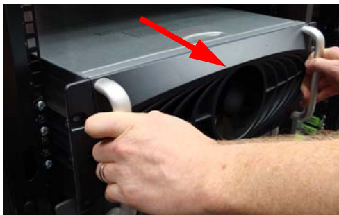
Figure 4.9: Sliding the unit forward in the rack
