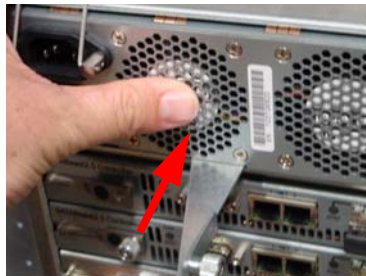
Figure 3.9: Sliding the PSU into place
