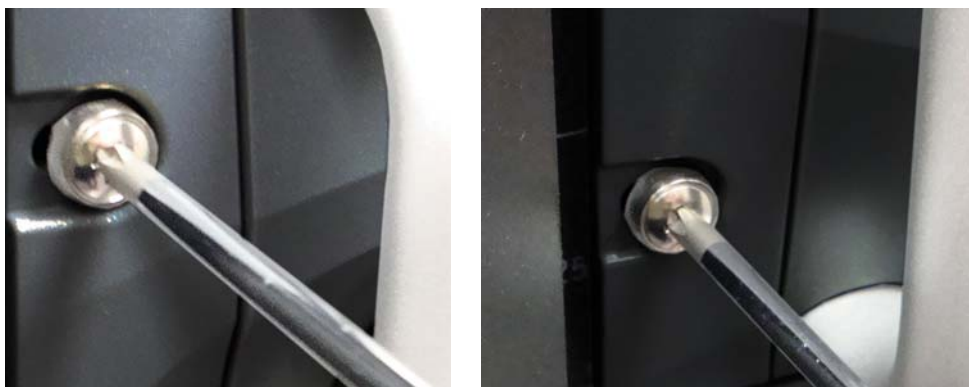
Figure 3.18: Bolting the SATABeast/SASBeast to the rack
