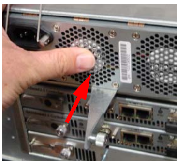
Figure 4.2: Sliding the PSU into place
