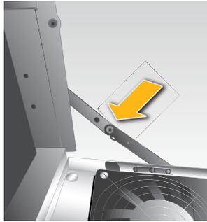
10. Raise the front panel and bolt it back into place.
