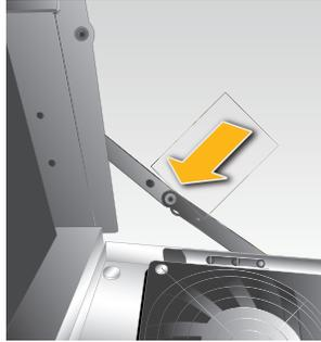
8. Raise the front panel and bolt it back into place.
