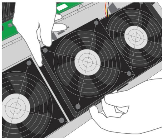
6. Snap the new fan in place and connect its power cord to the printed circuit board.
